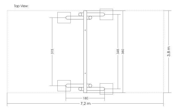
"Caution! Fences should have a distance of at least 1.5m from the lateral edge of the swing seat and 1.5m from the landing area in swinging direction according to a risk assessment. (DIN-EN 1176-2:2017-12 Appendix A)"
