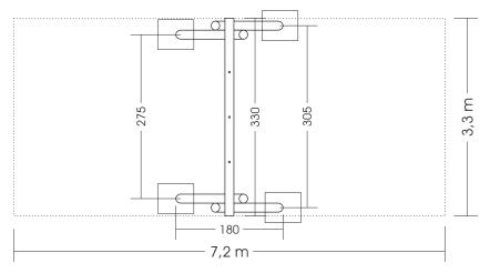
"Caution! Fences should have a distance of at least 1.5m from the lateral edge of the swing seat and 1.5m from the landing area in swinging direction according to a risk assessment. (DIN-EN 1176-2:2017-12 Appendix A)"
