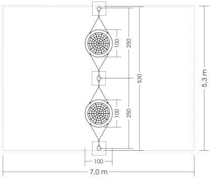
"Caution! Fences should have a distance of at least 1.5m from the lateral edge of the swing seat and 1.5m from the landing area in swinging direction according to a risk assessment. (DIN-EN 1176-2:2017-12 Appendix A)"
