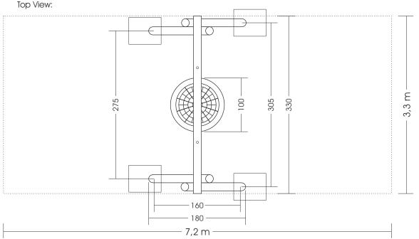
"Caution! Fences should have a distance of at least 1.5m from the lateral edge of the swing seat and 1.5m from the landing area in swinging direction according to a risk assessment. (DIN-EN 1176-2:2017-12 Appendix A)"
