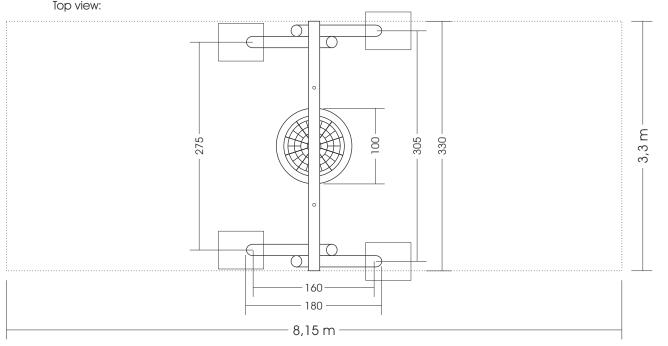
"Caution! Fences should have a distance of at least 1.5m from the lateral edge of the swing seat and 1.5m from the landing area in swinging direction according to a risk assessment. (DIN-EN 1176-2:2017-12 Appendix A)"
